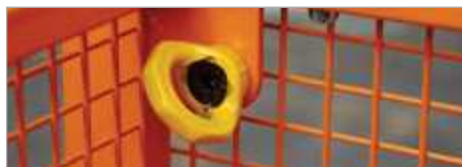
Anchorage point for protective equipment
